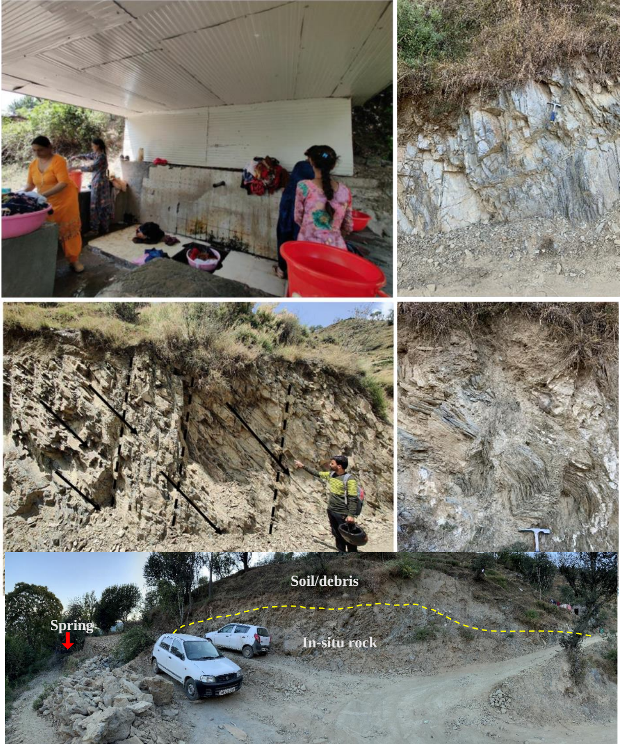
Fig. 5.36 Field photographs a) Springs RS-534 discharge point; b) phyllite in immediate vicinity of spring; c) locally exposed ( 32^{\circ}42'42.74''\text{N} , 76^{\circ}02'45.32''\text{E} ) slate with dip direction (arrows) and fractures (dotted lines); d) folding phyllite and e) synoptic overview of the area with visible contact between debris and rock.
